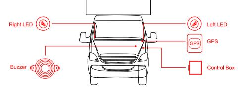
e.The warning light will be lit if the target vehicle in LCA detection area will overtake the vehicle within 5 seconds.
