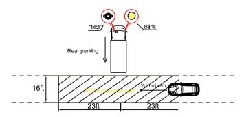
b.The warning light will be lit if there's relatively stationary target vehicle(Vo=Vs) in BSD detection area
