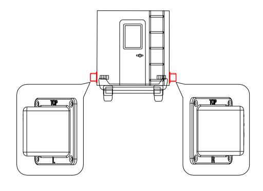
Use screw to fix sensors after select the correct installation position, make sure that sensor's installation side is parallel to vehicle body and fix cables with cable tie.
