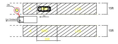
d.lf LED lit, and then turning signal was triggered, LED will blink; the buzzer will give out "bibi" warning beep.
